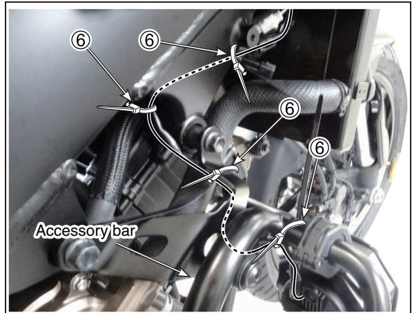
12.[Left side] Pass the harness of the LH LED lamp ① through the back of the Accessory bar A and the radiator hose, and temporarily fix the harness to the Accessory bar A in 2 points by using the Clamp ⑥.
