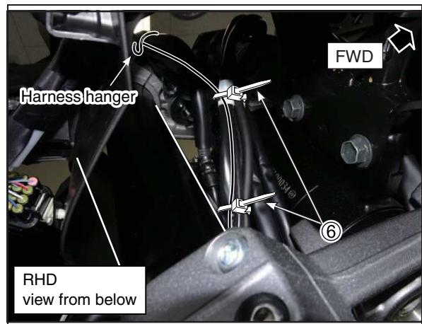
9. Pass the harness of the Switch ③ to the back of the radiator hanger along STD harness. (Connector will be connected in step (16))
