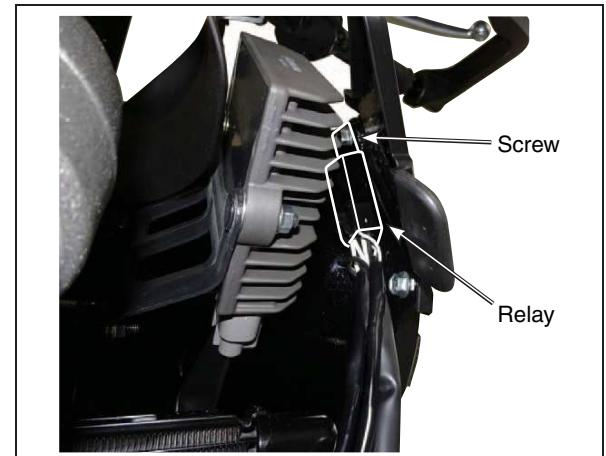
5. Pass the power source harness, switch harness and RH lamp harness of the Relay harness set ② from below the front left side of the fuel tank to the front right side of the vehicle through the front center bracket.
