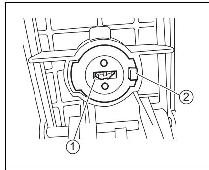
4. Apply a thread lock cement to the TORX® screws ① and install the lock plate ② by tightening the screws.
