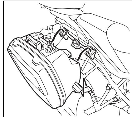
8. Fold the handle down and make sure that the locking bar ① is fit into the slot of the side case upper bracket.
