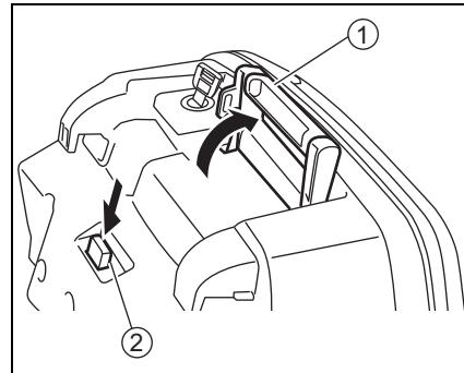
7. Install the side case onto the brackets as shown.
