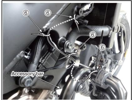
12.[Left side] Pass the harness of the LH LED lamp ① through the back of the Accessory bar A and the radiator hose, and temporarily fix the harness to the Accessory bar A in 2 points by using the Clamp ⑥.
