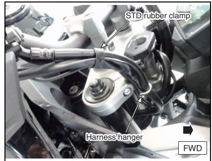
8. Pass the harness of the Switch ③ along STD harness around the RH front fork. Temporarily fix the harness to STD harness in 2 points by using the Clamp ⑥.
