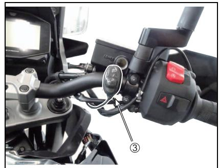
7. Pass the harness of the Switch ③ along STD harness through harness hanger and fix the harness by using STD rubber clamp.
