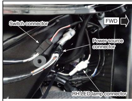
17.Make sure that RH/LH LED lamp and lighting devices of the bike operate normally.
