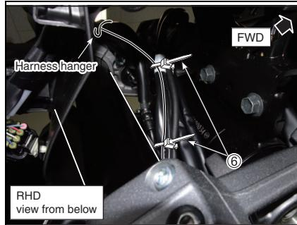
9. Pass the harness of the Switch ③ to the back of the radiator hanger along STD harness. (Connector will be connected in step (16))
