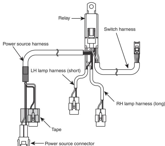
4. Remove upper screw of the LH front side inner cover and install the relay of the Relay harness set ② by using upper screw.
