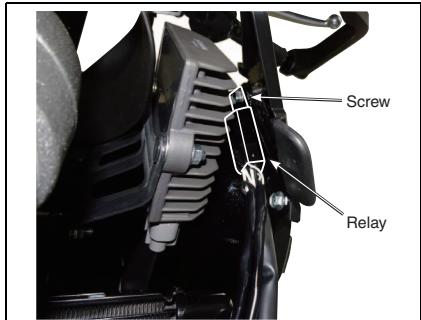
5. Pass the power source harness, switch harness and RH lamp harness of the Relay harness set ② from below the front left side of the fuel tank to the front right side of the vehicle through the front center bracket.
